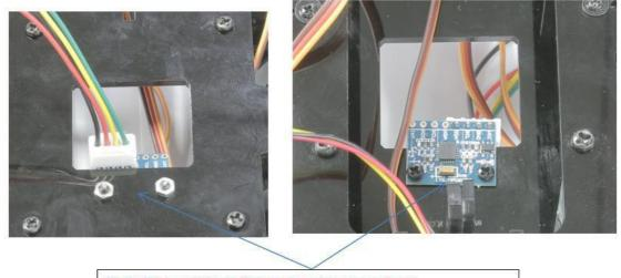
Note: The positions of the nut and screw are not interchangeable, otherwise the MPU6050 will be damaged.
