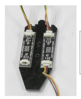
Note: The LED module has an input (IN) with a white edge and an output (OUT) without white edge. If the LED does not light up in yellow normally, then check if the input and output are reversed.
