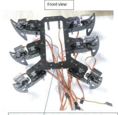
Note: The front of the bottom plate is without nylon standoffs. The legs on both sides should be as shown.
