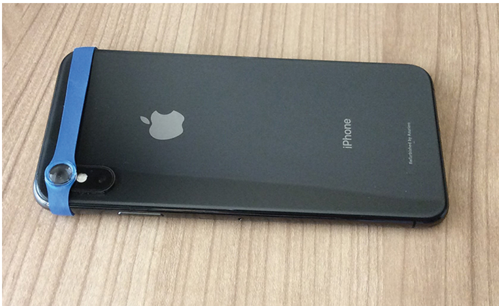
▲ FIGURE 4 Mounted appearance of a macro lens (Easy-Macro) to an iPhone XS Max. The flash component of many smartphones is aligned horizontally, rather than vertically, as shown here; this may obscure the flash and require the examiner to provide independent illumination (eg, penlight) to the eye.
