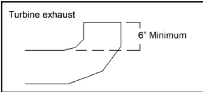
3. Exhaust stack diameter to be no smaller than 1 inch of engine outlet.
