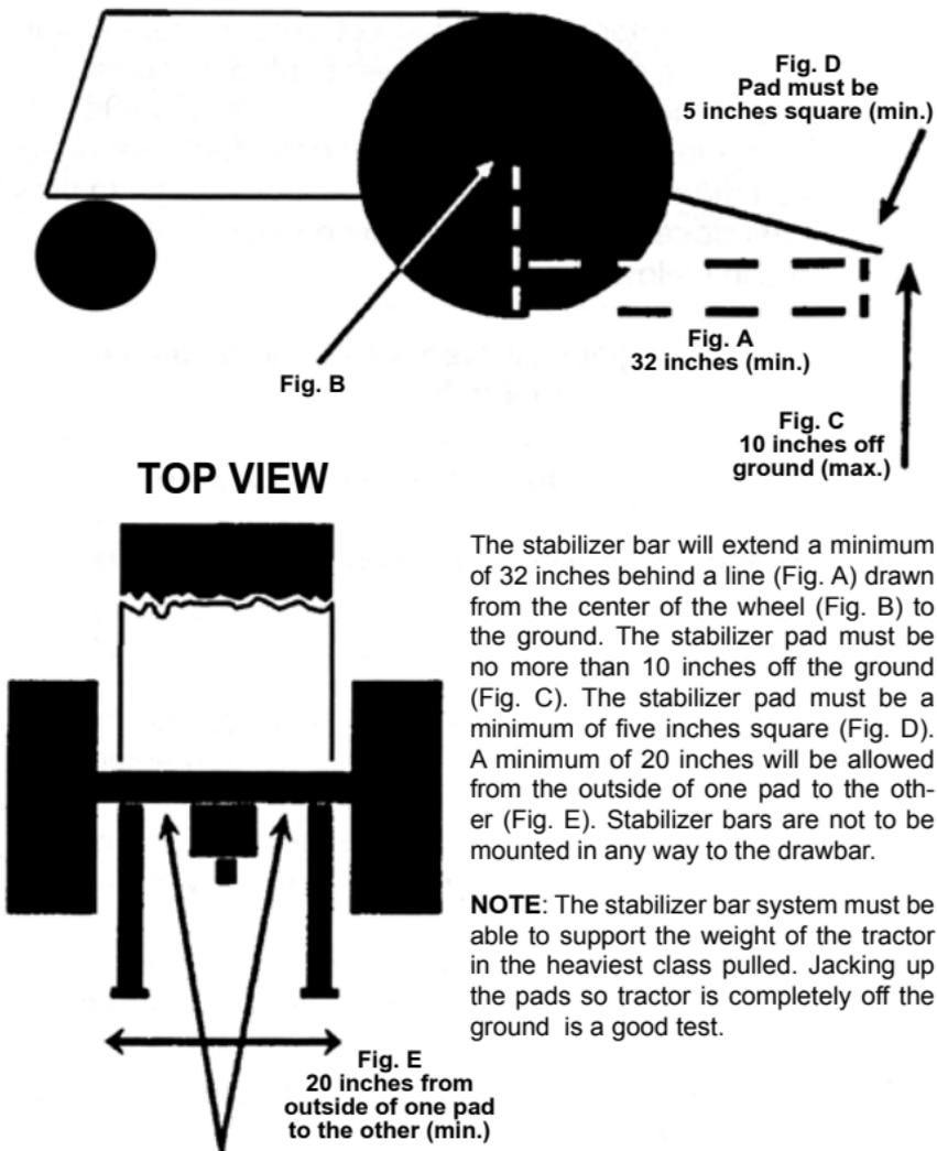
The stabilizer bar will extend a minimum of 32 inches behind a line (Fig. A) drawn from the center of the wheel (Fig. B) to the ground. The stabilizer pad must be no more than 10 inches off the ground (Fig. C). The stabilizer pad must be a minimum of five inches square (Fig. D). A minimum of 20 inches will be allowed from the outside of one pad to the other (Fig. E). Stabilizer bars are not to be mounted in any way to the drawbar.
