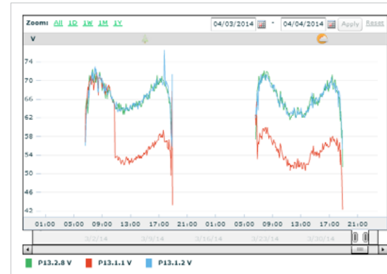
It is easy to identify the bypass diode failure with the module-level voltage graphs. The faulty module outputs at only 2/3 of the voltage (5/6 in this case of power optimizer connected to two modules).
