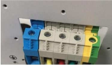
5.13 AC cable connected to the terminal
