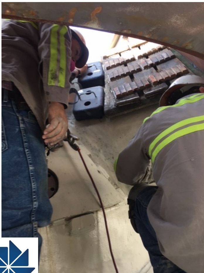
Installing Stronglock liners in the exposed area to protect gyratory crusher
