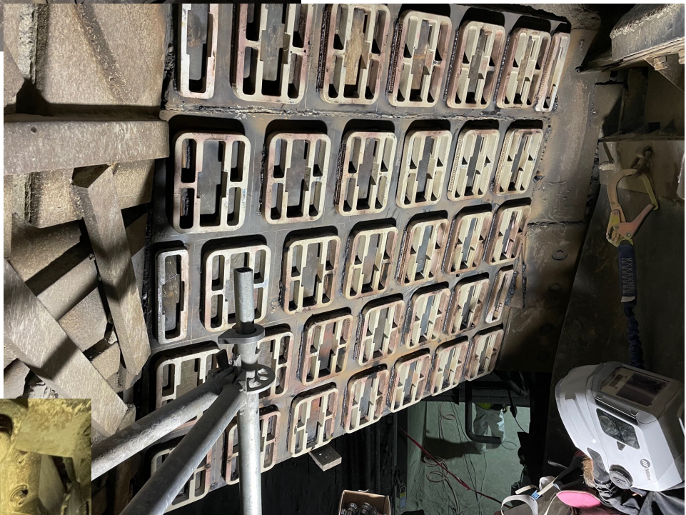
Wall repair under a Gyratory Crusher using the STRONGLOCK System
