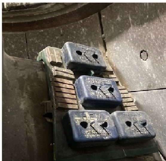
STRONGLOCK System implemented into high wear area which improved production from 1 year to 2 years
