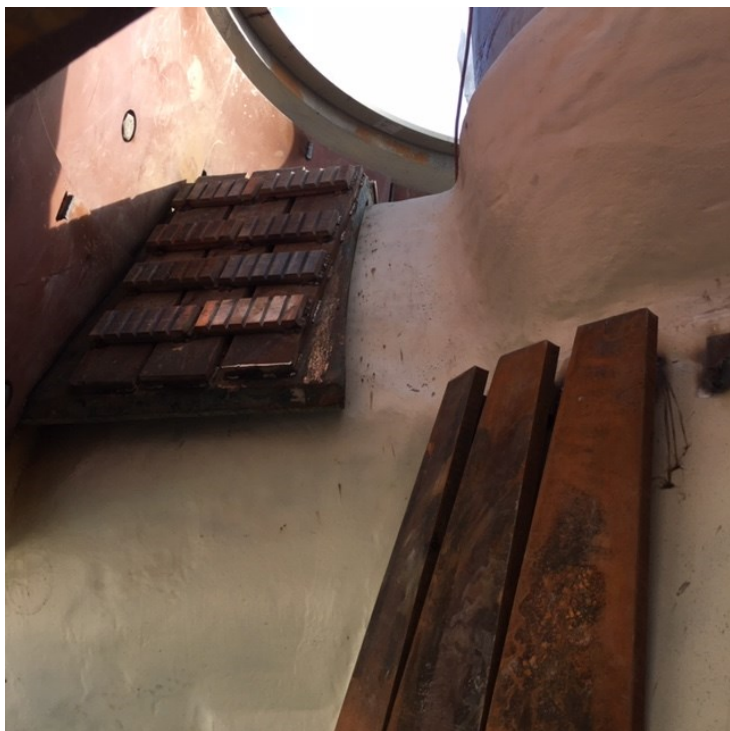
Installing Stronglock liners in the exposed area to protect gyratory crusher
