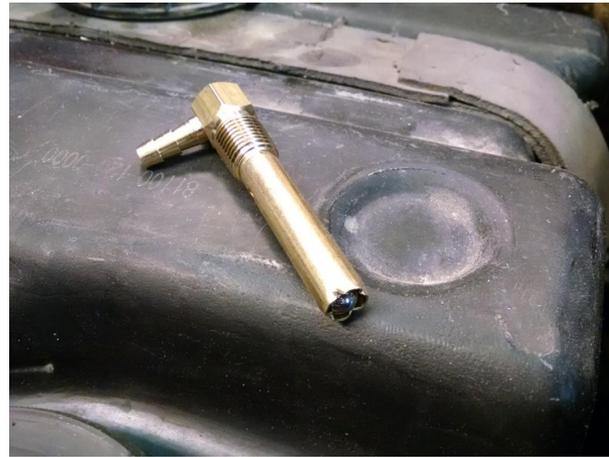
We then used a nice performance tubing from the new tank vent and routed it up and out of the way. We then re-installed the fuel pump assembly, making sure not to damage the OEM O' ring seal. Now when the unit should ever go over again, we do not have to fear fuel leaking onto the riders. This is an easy fix and runs about \$15.00 or so.
