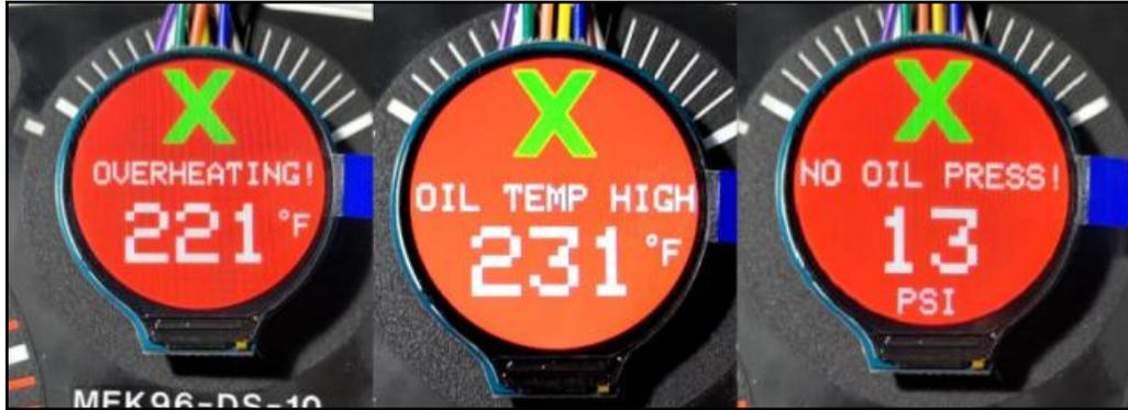
(please excuse the coolant one going off at 220F - the level was later raised to 225F/107C)
