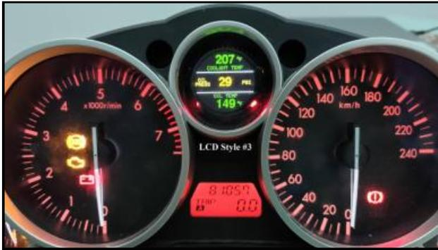
you overheat, the stock coolant gauge won't tell you until engine damage has occurred already. Add that on top of the infamous coolant bottle failure and it needs no more explaining. The exact position of the coolant temp. needle vs measured temperature can be customised to your liking.
