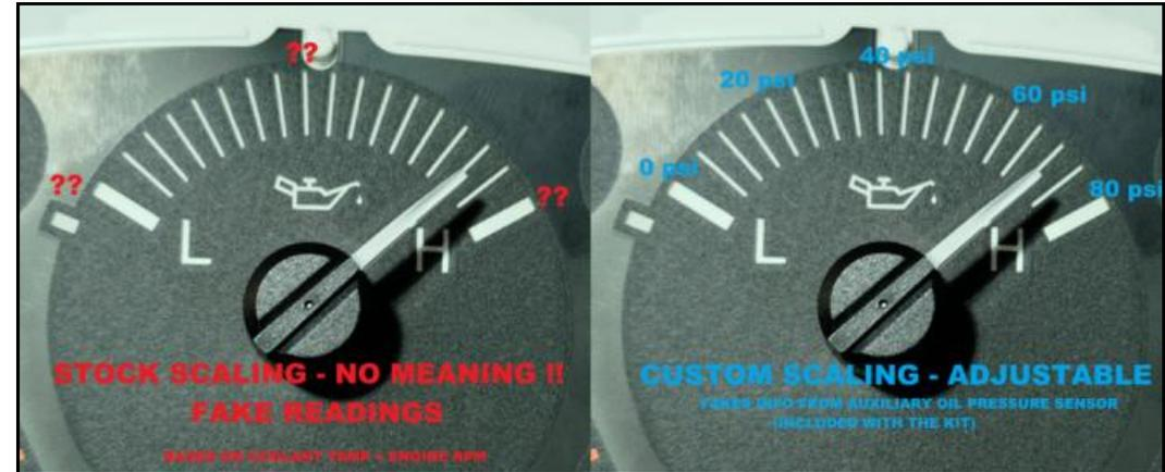
Now, for those of you that are more demanding there's the option of ditching the stock oil pressure gauge and installing a small screen in that area. That option will require a bit more DIY and taking the entire cluster apart, but the results will be worth it.
