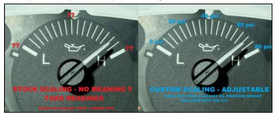
Now, for those of you that are more demanding there's the option of ditching the stock oil pressure gauge and installing a small screen in that area. That option will require a bit more DIY and taking the entire cluster apart, but the results will be worth it.
