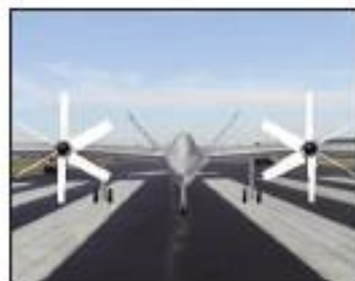
Outer propellers shown (90 degrees) fully turned. (Blainjett Aviation)
