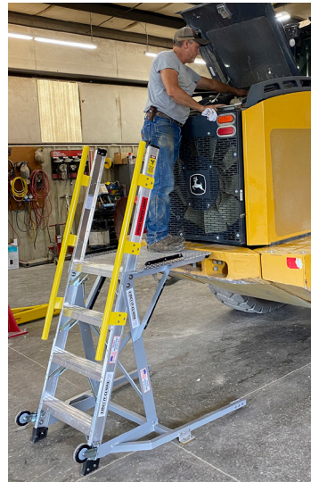
GRADERS servicing hoses, hydraulics, windshields, wipers, mirrors, lights, high engine components and other critical maintenance areas is safer and easier.
