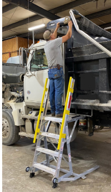
DUMP TRUCKS hard to reach and service areas can now be accessed in greater safety and comfort by using the 44" high rolling platform ladder stand.
