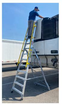
13LNCTRK is 13-feet tall and easily rolled by one person into position where the patented 6061-aluminum base extends out and locks into position. The ladder is then slid into position on replaceable brass and rubber feet. Three-point contact climbing is facilitated by the the yellow safety handrails.
