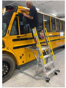
44LNCTRKENG affords safe stable working access to all service points along the side and rear, including running lights, windshields, racks, etc.
