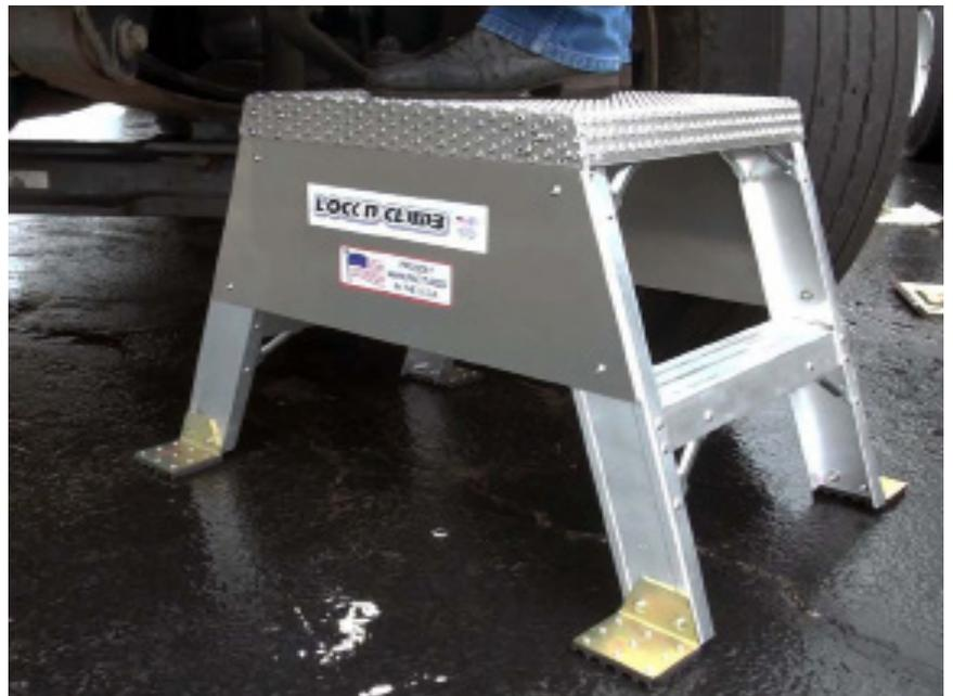
The 20LNCMINISTAND fits between the 44-inch tire and bumper and allows the maintenance technicians a stable slip-resistant platform to work on the truck engine rather than standing on slippery tires or struts. The 15LNCMINISTAND is employed when working on utility truck engines with 42-inch tires.
