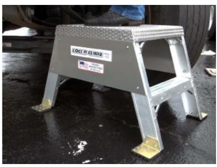
The 20LNCMINISTAND fits between the 44-inch tire and bumper and allows the maintenance technicians a stable slip-resistant platform to work on the truck engine rather than standing on slippery tires or struts. The 15LNCMINISTAND is employed when working on utility truck engines with 42-inch tires.
