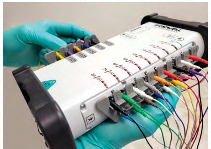
Quick Adaptors allow for fast and simultaneous connect and disconnect of groups of amplifier recording electrodes.
