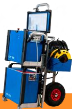
Brand: Omicron Model: CPC 100 & CP TD 1 Use: Primary Test System & Transformer Diagnosis
