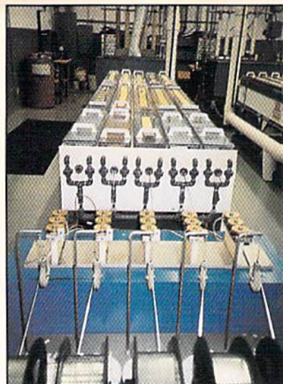
In a separate room at the plant, aluminum wires are anodized for use as voice coils in computers. This department can produce high-quality wire for the speaker industry.
