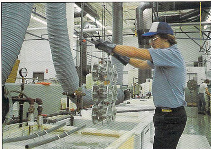
Internal motor drives for computer assemblies are carefully cleaned and treated prior to electroless plating. The shop environment is carefully controlled to ensure production of quality parts and employee safety. Note the corrugated blue pipes, which are super-high-velocity vents for carrying off any fumes released in the finishing process.
