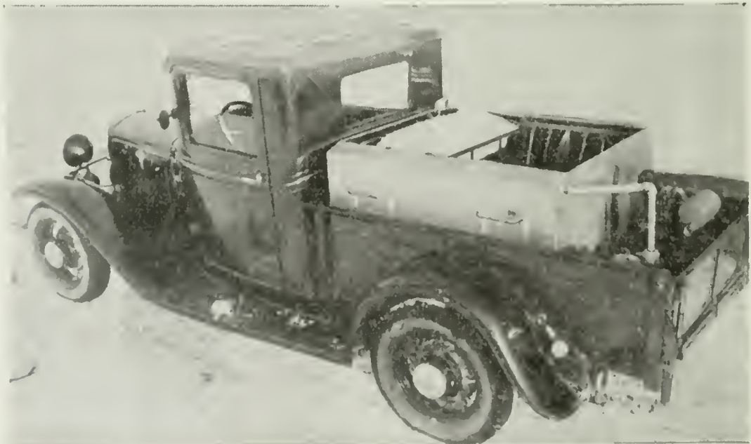
This new type of fish truck is now being used by the state fisheries division. With this apparatus for aeration, fish are taken many miles for planting, without loss.
