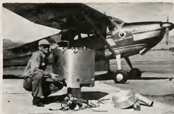
Pictured here is one type of tank used for aerial fish planting.
