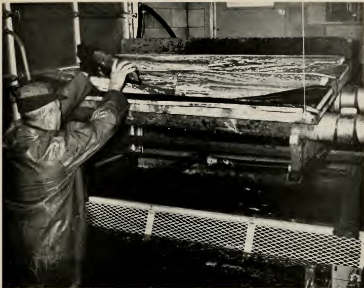
A unique trough, devised by Vern Campbell at the Arlee Hatchery, affords return of spawned fish to various raceways from a central spawning point.
