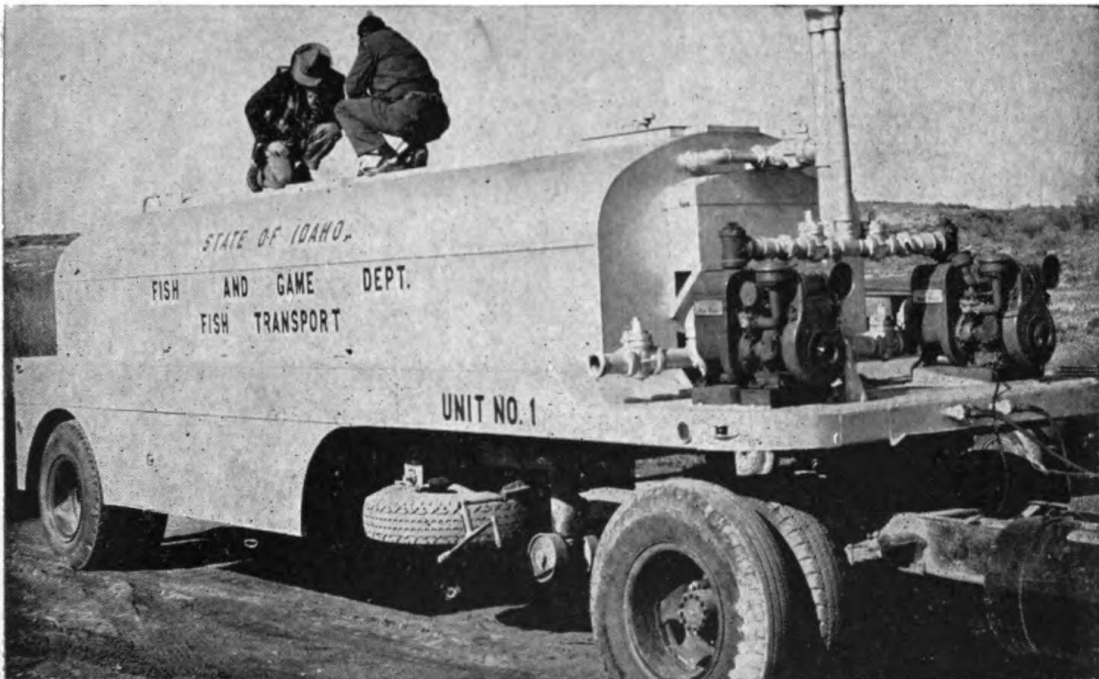
Huge tanker carries 1200 pounds of fish per load. Two of these transport units haul fish from Hagerman hatchery to northern sections of the state. Pumps at right keep water circulating in fine spray to provide fish with oxygen during their long road trip. Fish are rested for a day at McCall hatchery enroute north.
