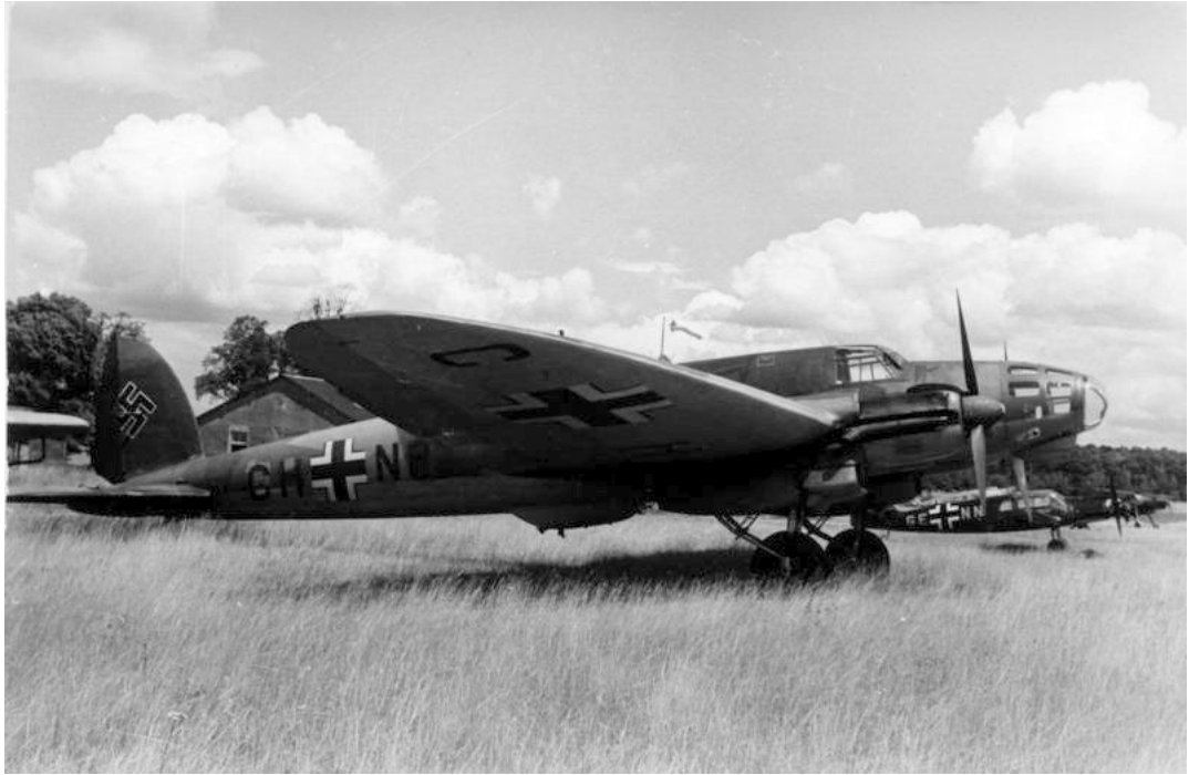
An He 111E in Luftwaffe service, 1940. The early variants had a conventional, stepped cockpit and the wings had a curved front edge: Bundesarchiv
