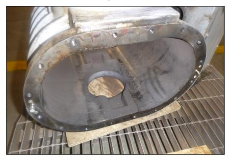
• Case is worn due to contact with the rotors. Case would need to be replaced with new.
