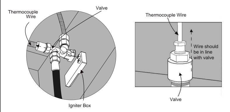
4. Make sure that the thermocouple wire is correctly positioned. The thermocouple wire should be in line with the valve.
