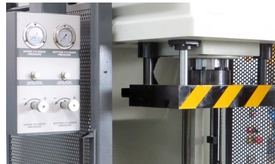
Hydraulic cylinder with cushion stroke (optional)
