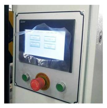
By displaying all press settings on a single screen, the touch screen control makes it easy to establish change, or
