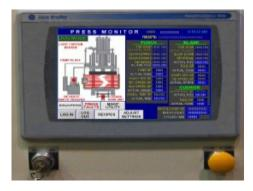
By displaying all press settings on a single screen, the touch screen control makes it easy to establish change, or verify set points. The Press Monitor screen lets you review actual stroke parameters and press performance while the press is in operation.
