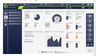
By displaying all press settings on a single screen, the touch screen control makes it easy to establish change, or verify set points. The Press Monitor screen lets you review actual stroke parameters and press performance while the press is in operation.
