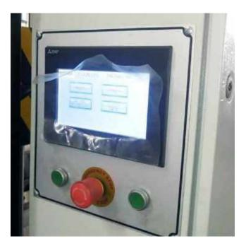
By displaying all press settings on a single screen, the touch screen control makes it easy to establish change, or verify set points. The Press Monitor screen lets you review actual stroke parameters and press performance while the press is in operation.
