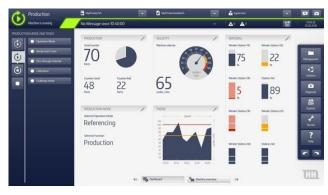
By displaying all press settings on a single screen, the touch screen control makes it easy to establish change, or verify set points. The Press Monitor screen lets you review actual stroke parameters and press performance while the press is in operation.
