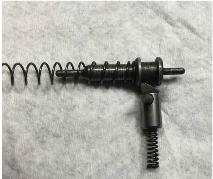
The later model safety will not allow the slide to be racked unless the safety is in the FIRE position. That doesn't mean the problem goes away – it just means a gun with a
