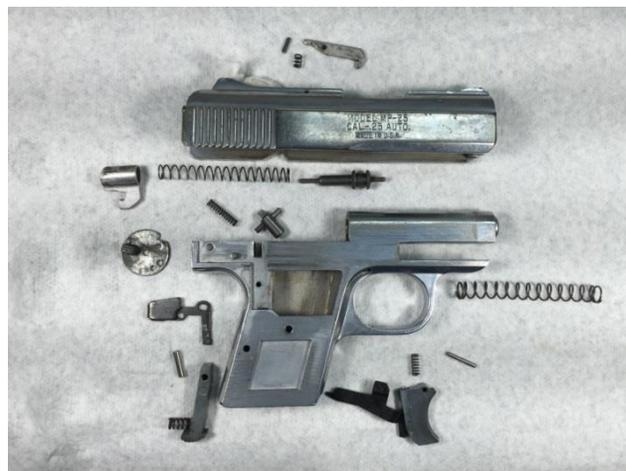
The Raven fire-control system consists of a single trigger bar and a disconnecter that is mounted externally on the right side of the frame. The sear and sear spring mount vertically in a well in the center of the frame. The disconnecter retains the sear and is itself retained by the right grip, which also keeps the trigger bar in alignment with the disconnecter. Without the grip, the trigger bar can slip outside the disconnecter.
