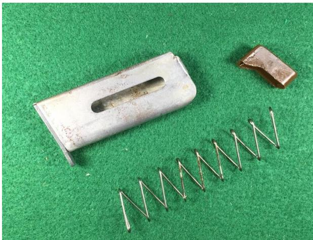
The Raven magazine can be disassembled, even though the base plate is staked on. You just need to depress and captivate the spring through the witness hole, then tilt the follower to take it out. After that, the spring comes out easily.
