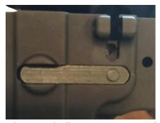
typical lower receiver shell. This is the way things are supposed to look, as I'm sure most of you have seen many times. It's a nice snug fit, with just enough clearance to let it slide straight out to release the magazine.
