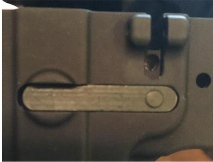
The next picture shows the magazine catch installed in the *customer's* gun, and now the problem is obvious. The slot in the lower receiver shell is cut too wide – not by much, just maybe a sixteenth of an inch or so – enough to let the catch pivot downward, allowing magazine to drop just enough that the bolt will miss picking up the next round.
