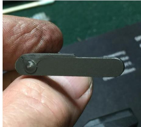
Filing and fitting took the most time, but I was pleased to note that the cured product matched the color of the part almost perfectly. Once installed (see picture below), the fix was almost invisible.
