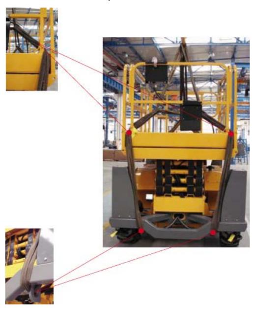
Procedure for the use of slings - Compact 10DX (Compact 2668RT) - Compact 12DX (Compact 3368RT) - Rear view of the machine
