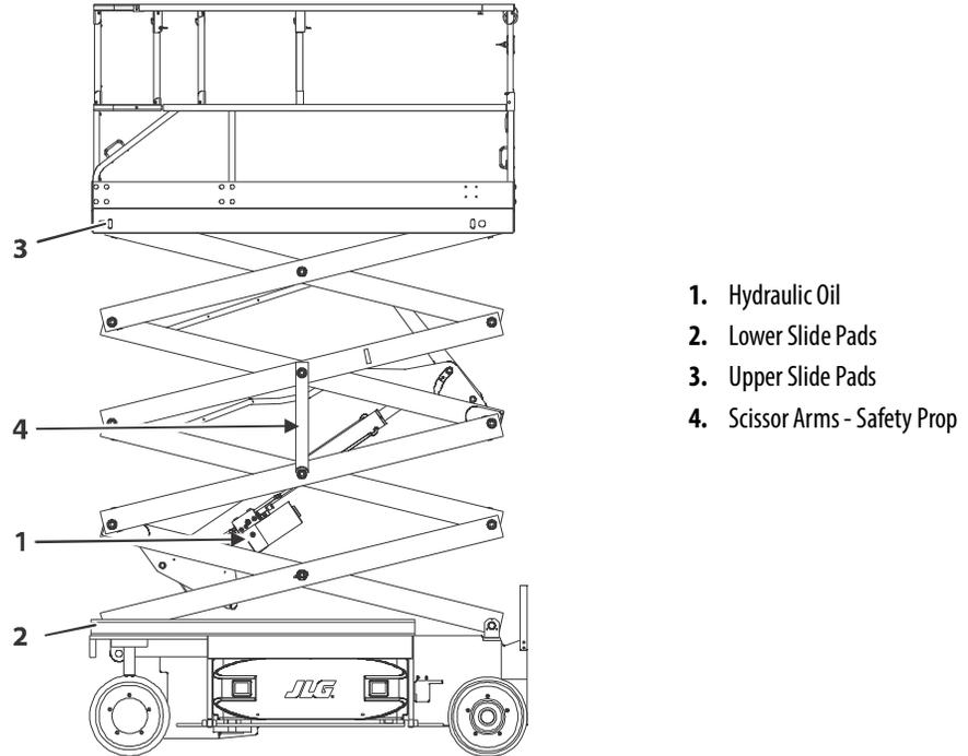
**Figure 6-1. Lubrication Diagram**
