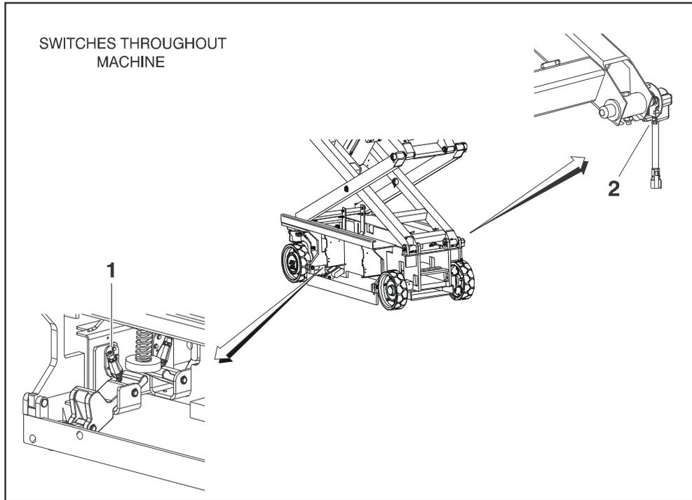
1. Pothole Switch (Typical on opposite side of machine)
