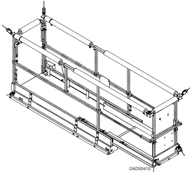
**NOTE:** Option with limit switches is shown.
