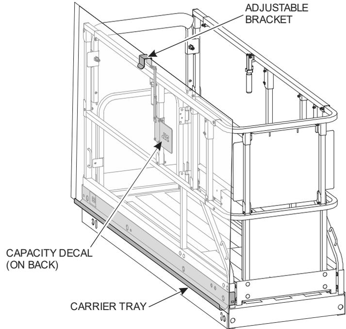
**NOTE:** Panel Carrier and Pipe Racks cannot be installed simultaneously if WorkStation is installed, although they are interchangeable.
