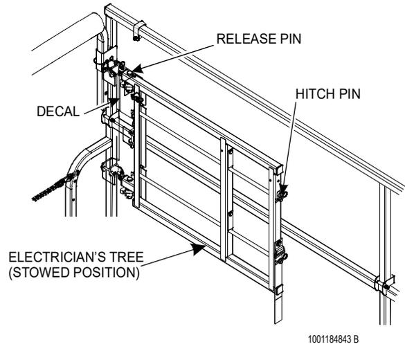
**NOTE:** *The Electrician's Tree may be simultaneously installed with Panel Carrier, Pipe Racks, QuikWelder, or WorkStation as long as it is mounted on the opposite side of the platform.*
