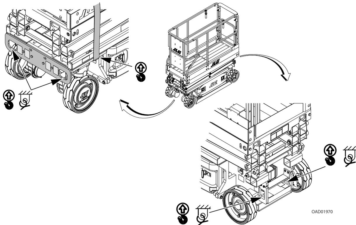
Figure 3-9. Lifting and Tie Down Diagram
