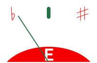
If the needle on the device is to the left, the string pitch is flat, meaning the note is lower than it should be. You'll need to raise the pitch.
