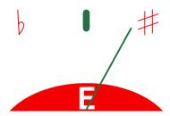
If the needle on the device is to the right, the string pitch is sharp, meaning the note is higher than it should be. You'll need to lower the pitch.
