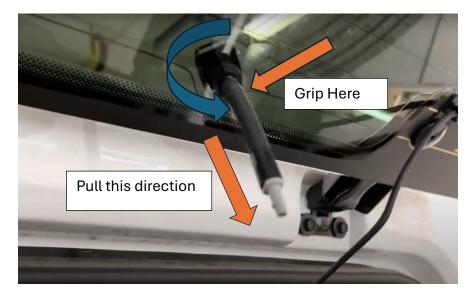
After pulling the hose off the nozzle, rotate the nut on the nozzle counterclockwise to remove the nozzle.
