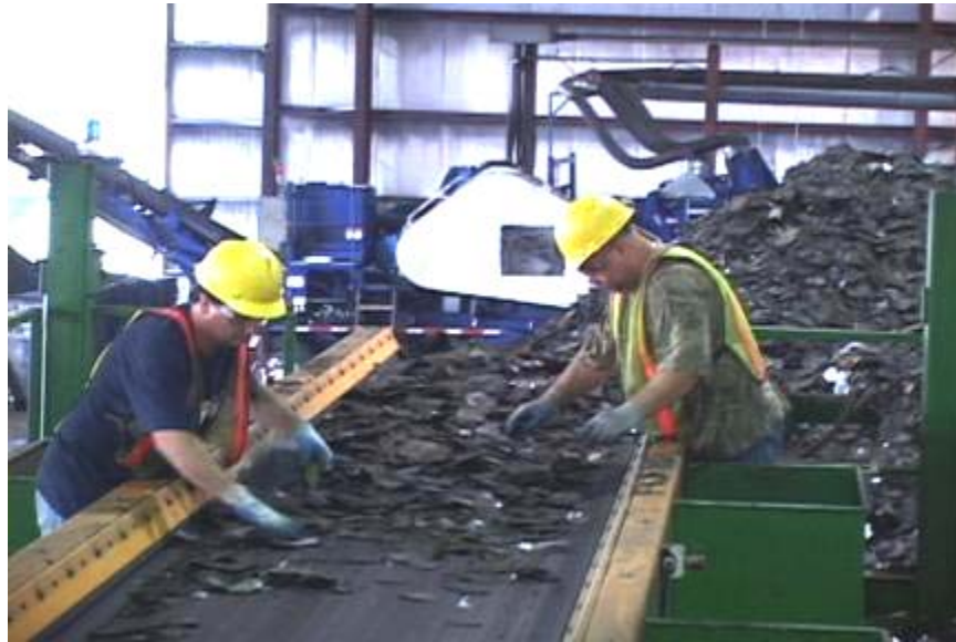
Picture 8 - Manual Sorting Stations on Elevated Platform Quality of sorted shingle product is affected by belt speed, burden depth, number of sorters, and sorters' performance.
