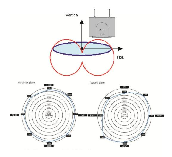
Figure 3.2.2-2 Antenna Radiation Pattern
