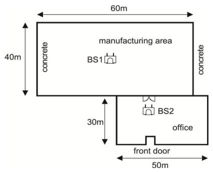
**Figure 3.2.4-2 Centralized Base Station Placement**
