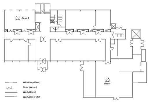
Figure 3.2.2-3 Sample Temporary Base Station Position
