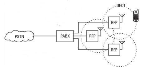
Figure 2.1 General DECT reference model of Wireless Office Terminal System
