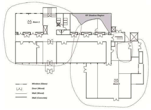
Figure 3.2.3-1 Cell Boundary Map with Base 1 and Base 2
