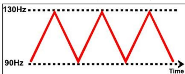
Most machines offer several sweep patterns, though there is very limited 'evidence' to justify some of these options. In the classic '**triangular**' sweep pattern, the machine gradually changes from the base to the top frequency, usually over a time period of 6 seconds – though some machines offer 1 or 3 second options. In the example illustrated, the machine is set to sweep from 90 to 130Hz
