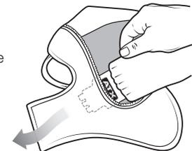
**4** Overlap the three wing-like pieces on one side of the Heat Exchanger. Insert the wing-like pieces into the corresponding side wing space of the Sleeve. The wings will remain overlapped in the provided space.
