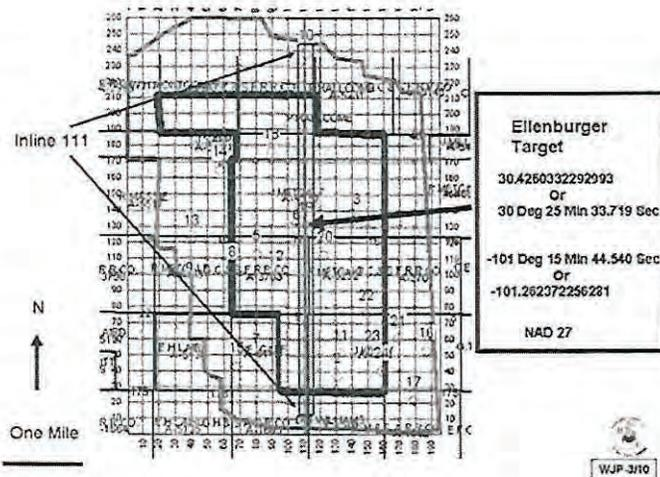
The north-south oriented 3D seismic inline #111 noted on the map is shown on the presentations at right and below. The 3D seismic presentations have been flattened on the base of the Ellenburger to accentuate the visual impact of the collapse zone. In each instance the standard seismic amplitude presentation is shown on the top of each picture, and the lower image illustrates that same section of seismic presented highlighting a different type of seismic attribute. In the case of
