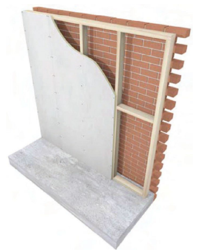
Figure 2.4. Masonry brick or block wall
