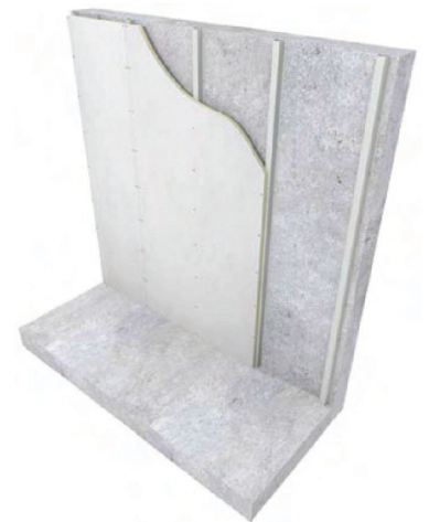
Figure 2.2. Masonry brick or block wall
