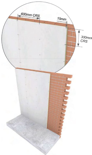
Figure 1.6. Masonry brick or block wall
