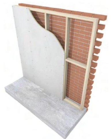
Figure 2.4. Masonry brick or block wall
