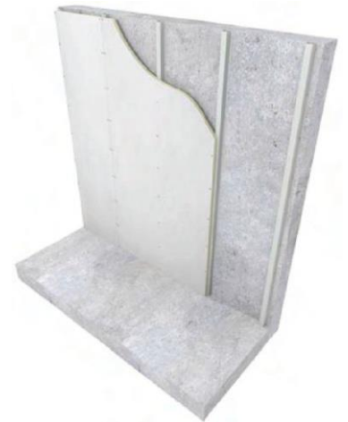
Figure 2.2. Masonry brick or block wall
