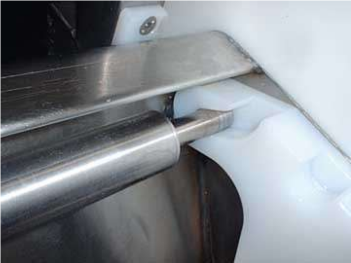
This picture shows the center fine adjuster (#26).
