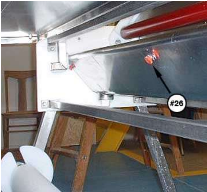
This picture shows the center fine adjuster (#26).
