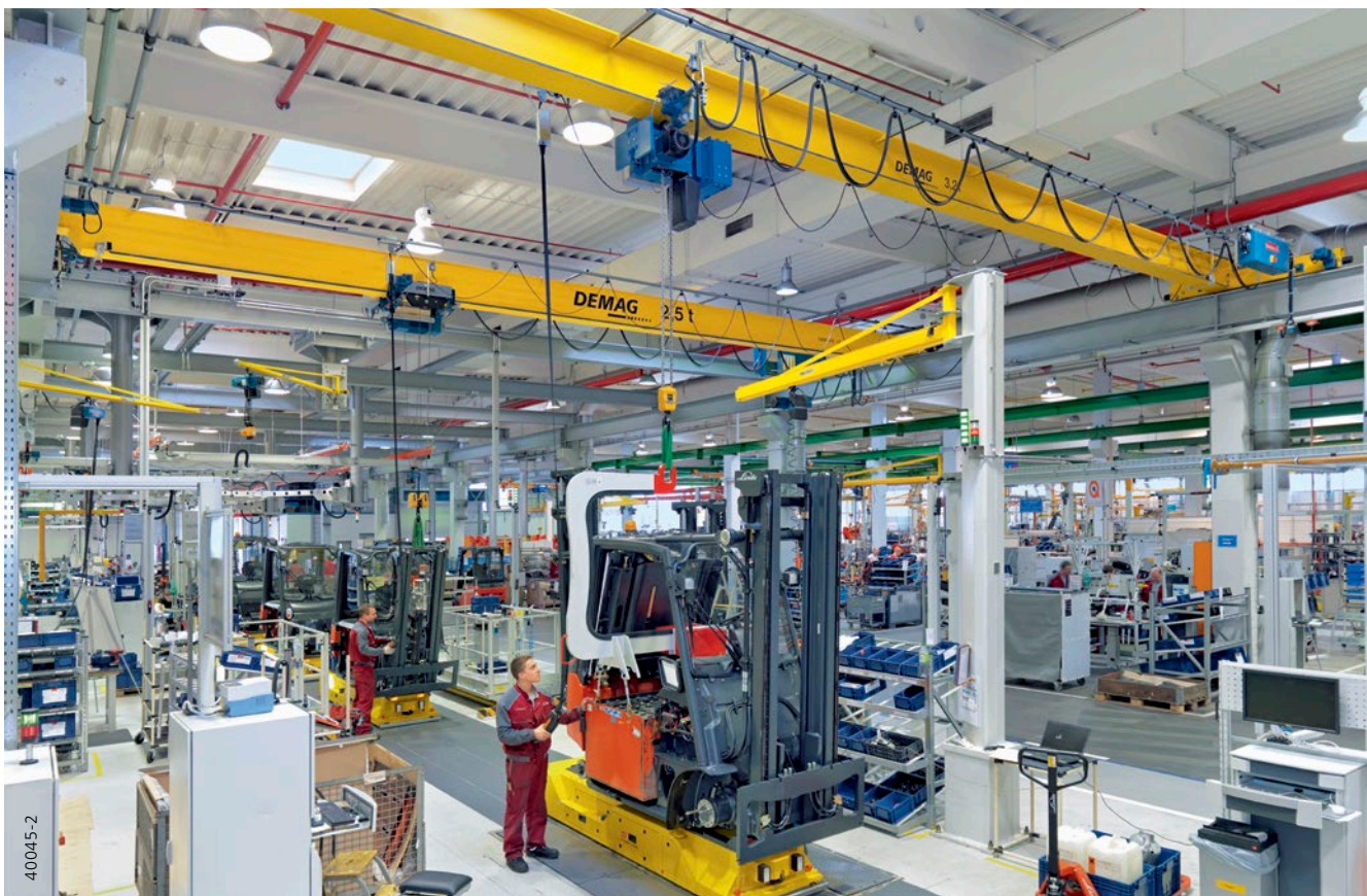
Assembly line for forklift trucks: Crane type EPKE equipped with DC chain hoist
