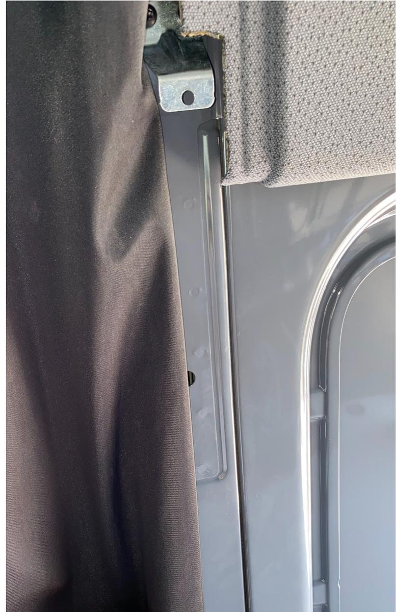
10. Secure the screen door on the front end of the van by using another plastic strip along with the  $\frac{3}{4}$ " self tapping screws to the B-pillar of the van as shown in Fig 2.22. Try to keep the magnets as vertical as possible when securing this area of the screen to the B-pillar.
