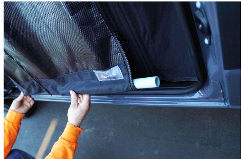
4. Clamp the screen to the top of the pinch weld of the van. Adjust the screen so that there's roughly only a ¼" gap between the screen and the floor and try to keep the middle zipper as centered to the opening as possible. You can use the brake light and backup camera as a point of reference (Fig 3.4).
