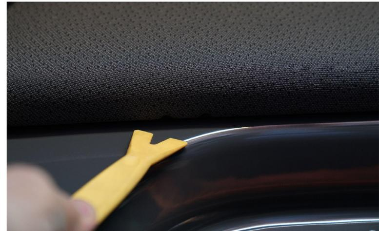
6. Once step 4 is complete, move toward the center of the middle ceiling panel where it meets with the rear ceiling panel (fig 2.4). There are several plastic clips holding the panel to the ceiling frame - gently pop these out with the panel pullers to release.
