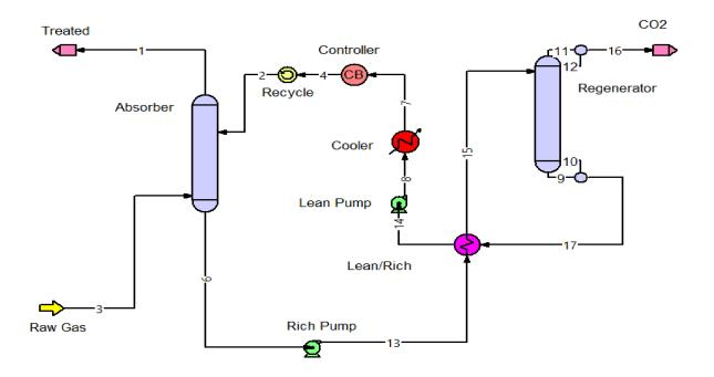
Fig.4.2 Process Flow Sheet (MEA Generic Valve Trays Without Wash Section)
