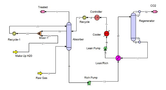
Fig.4.1 Process Flow Sheet (MEA Generic valve Trays with Wash section)
