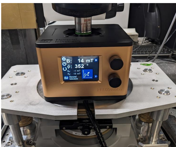
Figure 2: FLUXmoto into a MOKE microscope (left), replacing the electromagnet, power supply and water chiller. Optical microscope image of a sample under investigation with the FLUXmoto augmented MOKE (right).
